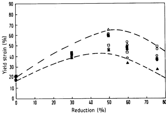
Figure 13 Variation of yield strain with percentage reduction. Orientation angle: (○) 0°, (●) 10°, (○) 20°, (■) 30°, (□) 45°, (▲) 60°, (△) helix angle.
