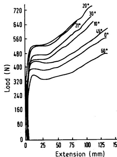
Figure 7 Load–extension curves for specimens flow-formed to 50% reduction.
