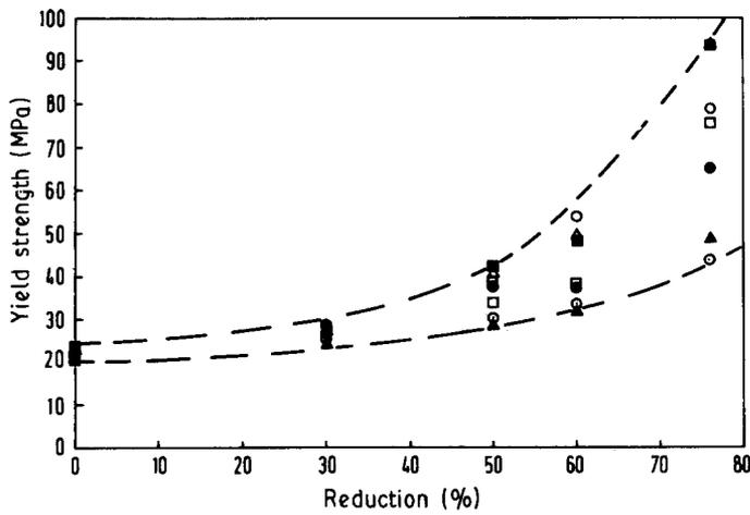
Figure 11 Variation of yield strength with percentage reduction. Orientation angle: ( $\circ$ ) 0°, ( $\bullet$ ) 10°, ( $\circ$ ) 20°, ( $\blacksquare$ ) 30°, ( $\square$ ) 45°, ( $\blacktriangle$ ) 60°, ( $\Delta$ ) helix angle.
