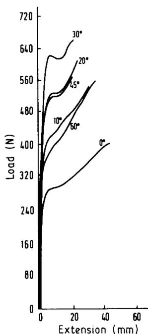
Figure 9 Load-extension curves for specimens flow-formed to 76% reduction.
