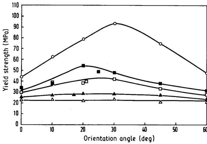
Figure 10 Variation of yield strength with orientation angle. Reduction: ( $\Delta$ ) 0%, ( $\blacktriangle$ ) 30%, ( $\square$ ) 50%, ( $\blacksquare$ ) 60%, ( $\circ$ ) 76%.
