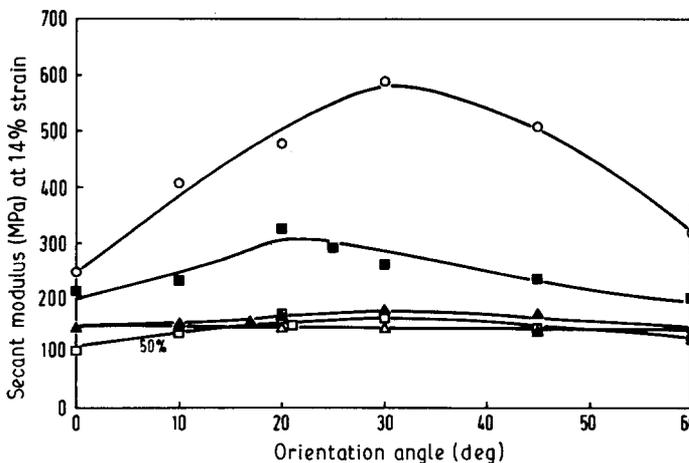
Figure 12 Variation of secant modulus with orientation angle. Reduction: ( $\Delta$ ) 0%, ( $\blacktriangle$ ) 30%, ( $\square$ ) 50%, ( $\blacksquare$ ) 60%, ( $\circ$ ) 76%.
