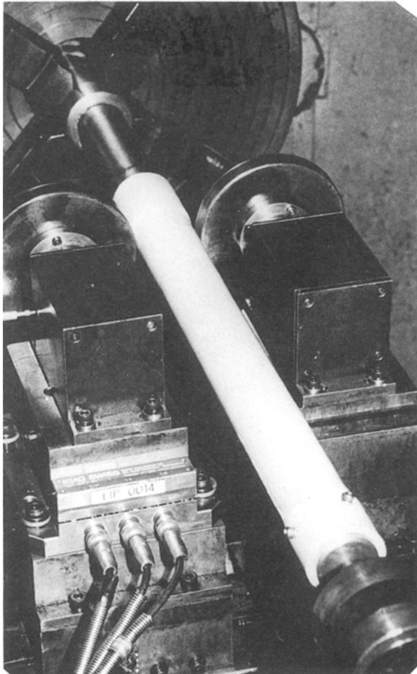
Figure 3 Experimental set-up for two-roller forward flow-forming process on a lathe.
