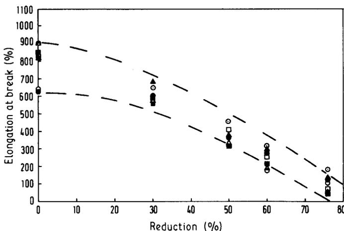
Figure 15 Variation of elongation at break with percentage reduction. Orientation angle: (○) 0°, (●) 10°, (○) 20°, (■) 30°, (□) 45°, (▲) 60°, (△) helix angle.
