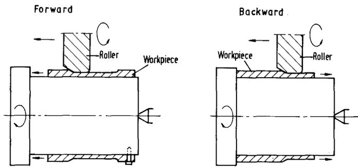
Figure 1 Schematic drawing of the forward and backward flow-forming processes.
