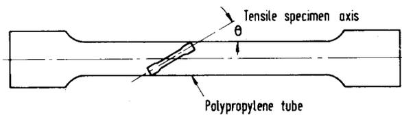
Figure 4 Definition of orientation angle.
