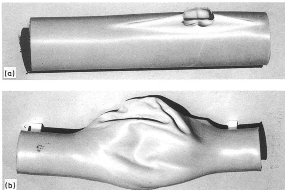
Figure 2 Pressure rupture behaviour of (a) an unflow-formed pipe, and (b) a flow-formed pipe showing ductile mode of rupture.
