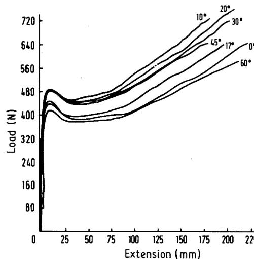
Figure 6 Load–extension curves for specimens flow-formed to 30% reduction.
