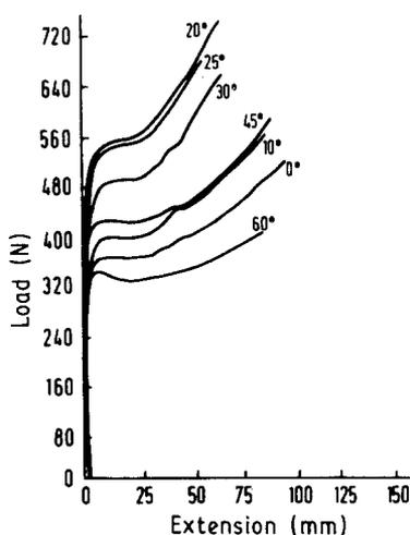
Figure 8 Load-extension curves for specimens flow-formed to 60% reduction.
