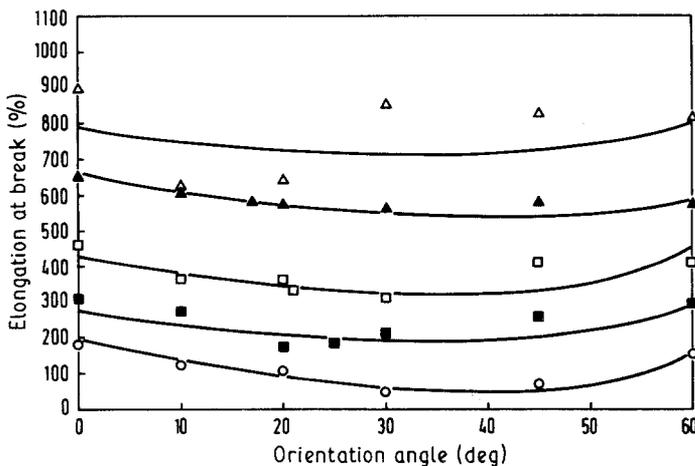
Figure 14 Variation of elongation at break with orientation angle. Reduction: (△) 0%, (▲) 30%, (□) 50%, (■) 60%, (○) 76%.
