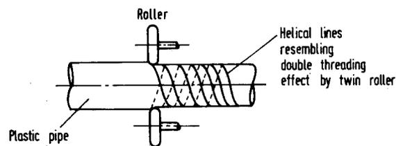
Figure 5 Schematic drawing illustrating the formation of helical lines during the flow-forming process.
